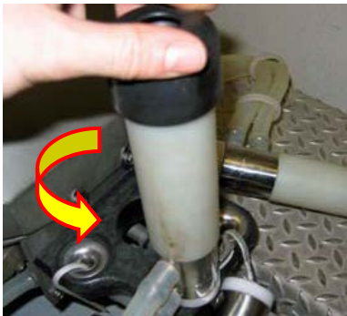
1. Rotate shell anti clockwise and remove
