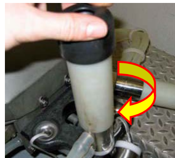
6. Screw the shell back into the milk vacuum chamber; ensure that the liner is not twisted.
