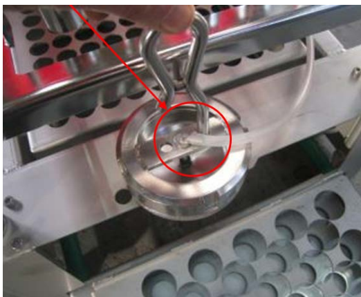
Connect the other end of the sampler 'D' tube to the spoon on the sampler
