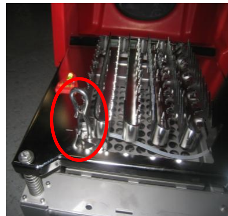
Place the spoon into position 1 of the toothed section. Ensure that the silicone tube is routed so that it cannot catch on an obstruction.
