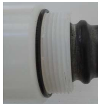
4. Fit new liner and pull into shell as far as shown (middle groove).
