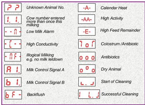
If Milking is Blocked (display shows STOP or -nF-) due for example to an animal being Dry or has Antibiotics then press the OK key to acknowledge the warning and then press the START key once more
