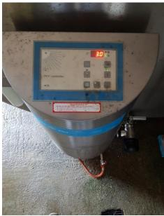
After Milk Collection, Press and Hold 1 until you hear click and water drain Only turn on when ready to start milking Then press and hold 2 until green light beside 3 starts flashing 10 minute delay from time you turn on tank to when it turns on
