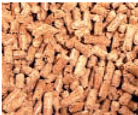
Sawdust is compressed through a die under high pressure and temperature producing wood pellets
