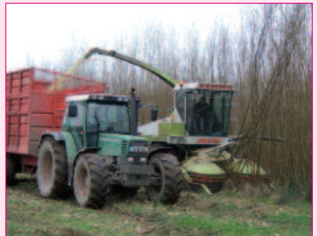
Forage harvester with adapted maize head harvesting willow
