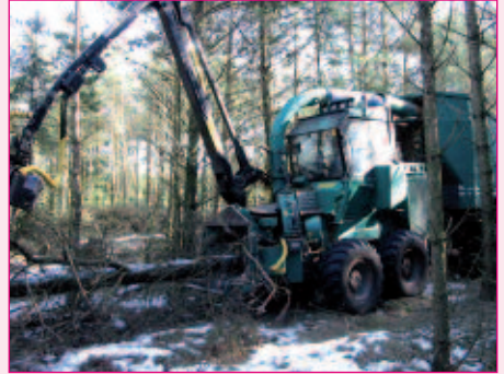
Harvesting machine chipping wood in the forest.
