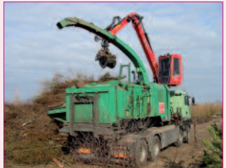
Wood can also be chipped at the roadside using a mobile chipper.
