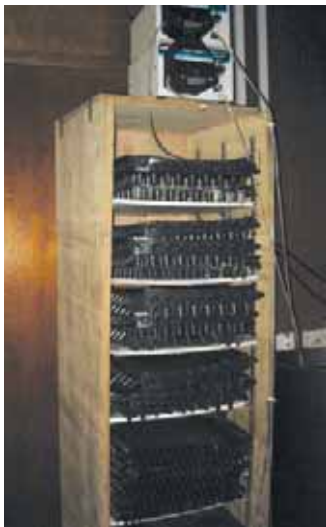
This horizontal flow biofilm reactor (HFBR) device was developed at NUIG for the treatment of synthetic wastewaters.
