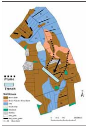
Contamination migration intercepted by denitrification trench.
