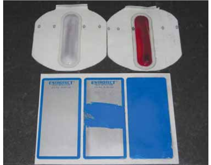
FIGURE 2: Top: inactivated (left) and activated (right) Check Mate® devices. Bottom: inactivated (left), partially activated (middle) and completely activated (right) EstroTECT™ heat detectors.
