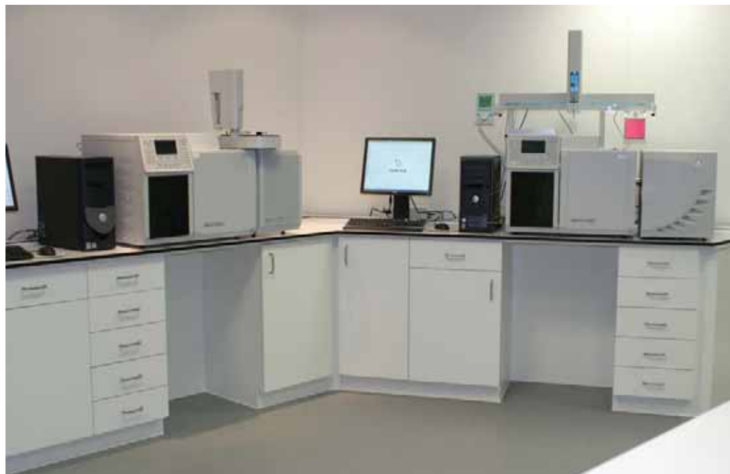
Varian 3800 GC with cryogenics and flame ionisation detector and Varian 3800 GC with multi injection Combi PAL autosampler, cryogenics and Varian Saturn 2000 mass spectrometer.
