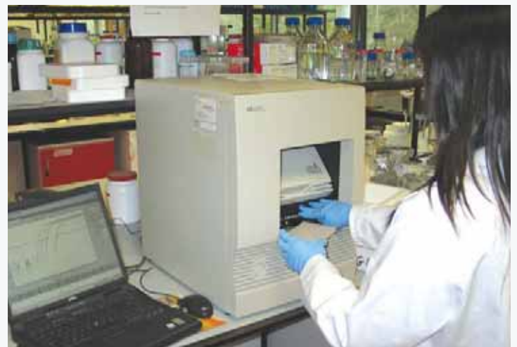
Using real time PCR facilities at Oak Park to examine the gene expression profiles of candidate genes for abiotic stress tolerance.
