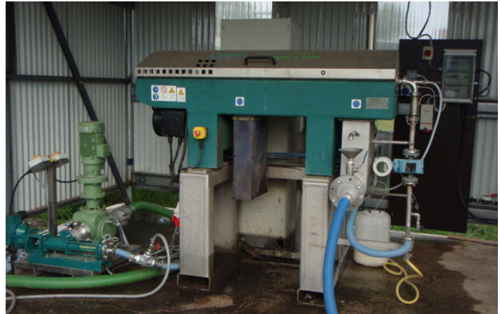
A fixed decanter centrifuge
