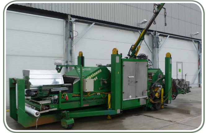
4. Head filling machines should be cleaned thoroughly before use, as fragments of infected compost can cause problems
