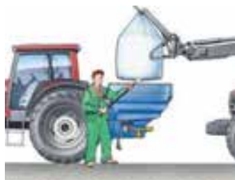
Use a knife with a long handle to cut the bag. Never walk under suspended load.
